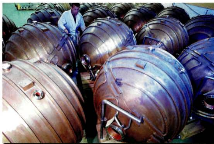
Looking rather as if surrounded by a collection of ornate urns, a technician surveys copper-accelerating cavities used in LEP. From 1996 these were gradually replaced by superconducting cavities that were to double the total collision energy from 100 GeV to just over 200 GeV.
