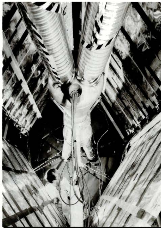
The Intersecting Storage Rings (ISR), the world's first proton-proton collider, started up in 1971, and later provided the first proton-antiproton collisions and the first collisions of beams of heavier ions (alpha particles). This image shows the vacuum chamber at one of the points where the proton beams crossed in the ISR.
