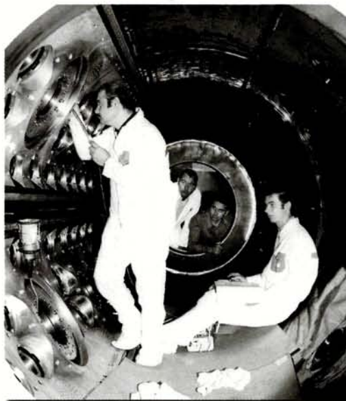
Assembly in progress inside the Gargamelle heavy-liquid bubble chamber, which was built at Saclay in France and came into operation at the PS in 1971. The chamber had a cylindrical body 4.8 m long and 1.85 m wide, with a volume of 12 cubic metres.
