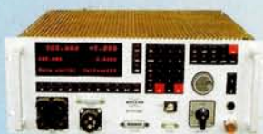
5V/300A for supraconducting magnets with 10 extra shims
