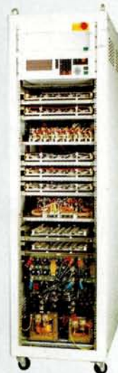
80V/600A, 50kW linear technology < 5ppm stability IEE488
